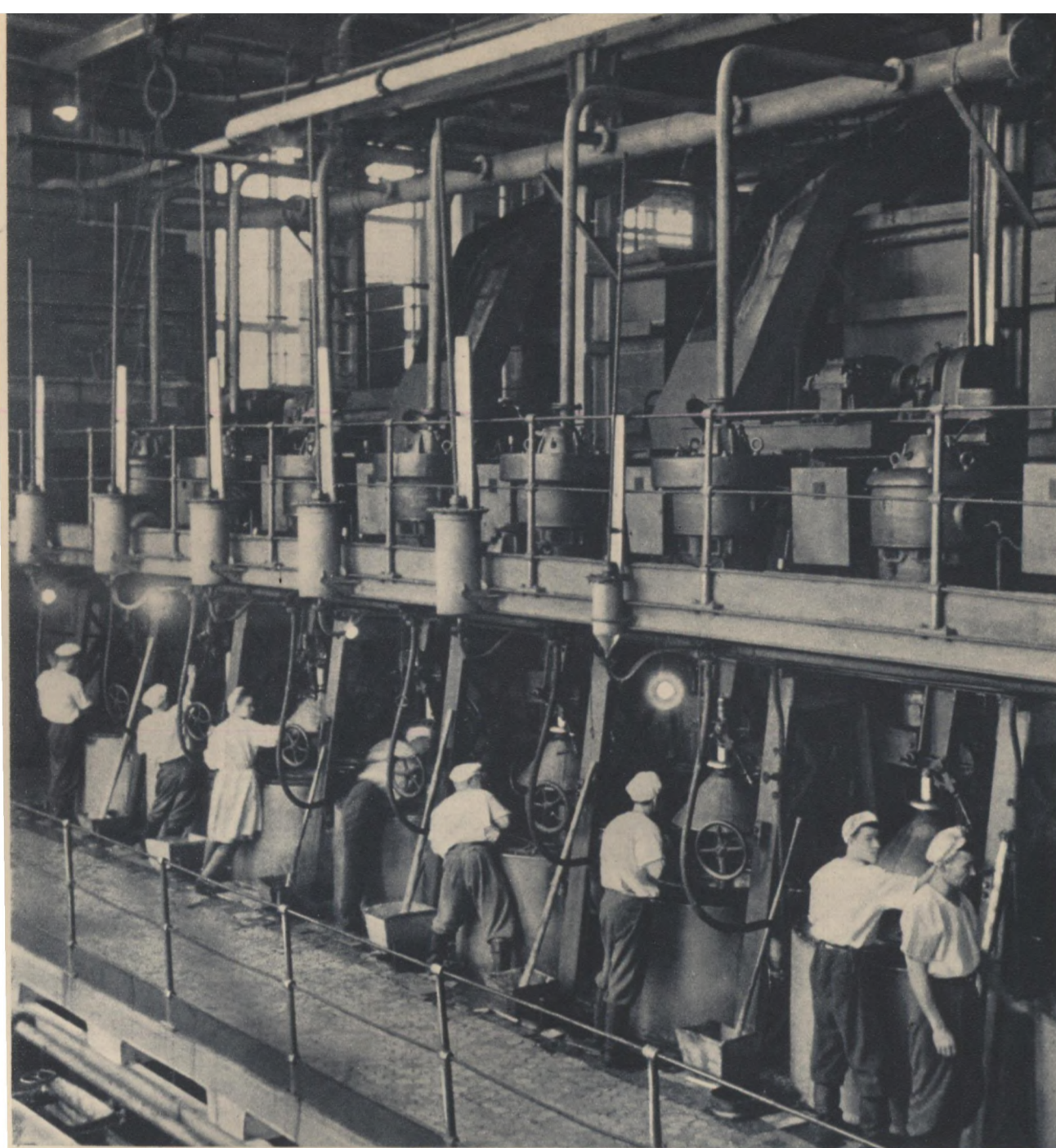
These centrifugal machines separate sugar crystals from the liquid sugar
