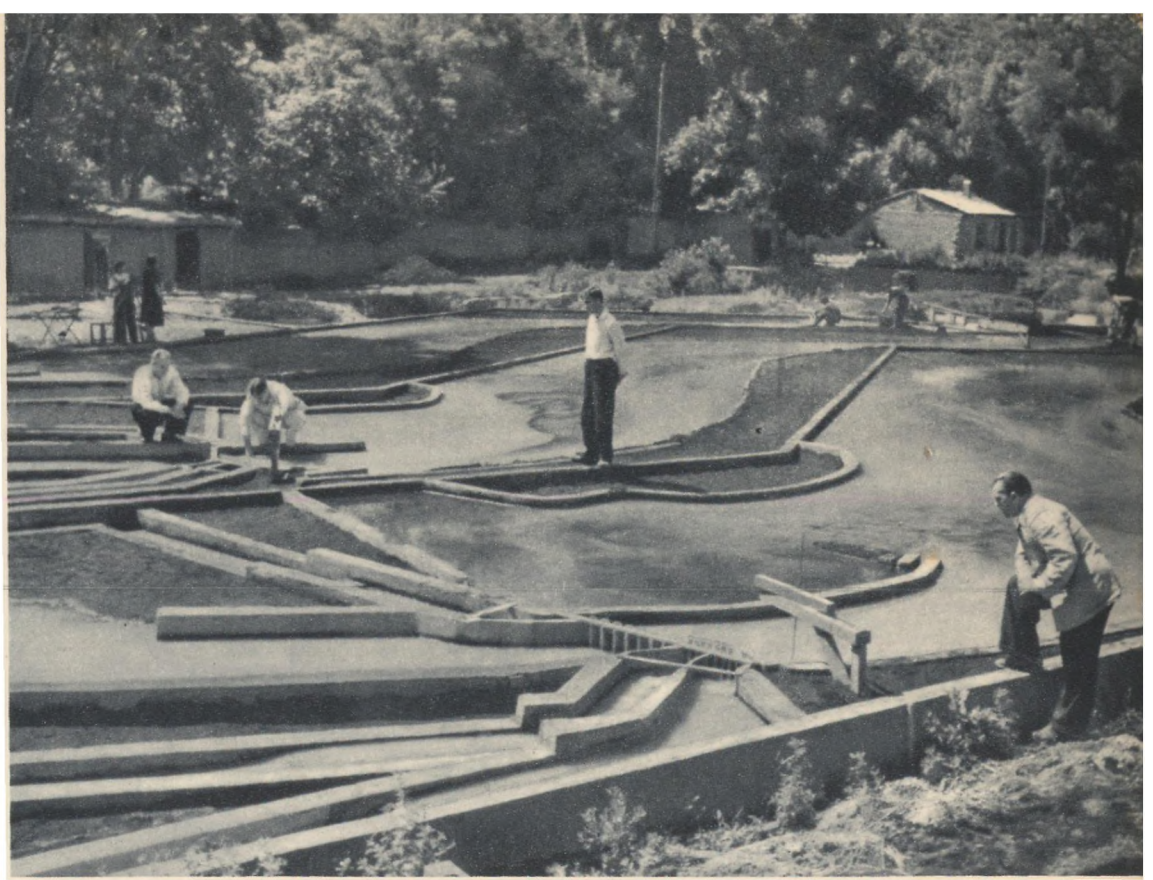
TASHKENT. Models of future structures on the Main Turkmen Canal are being studied at the Central Asian Irrigation Research Institute. Here we see a model of the Tahla-Tash network undergoing tests Photo by G. PERMENEV
