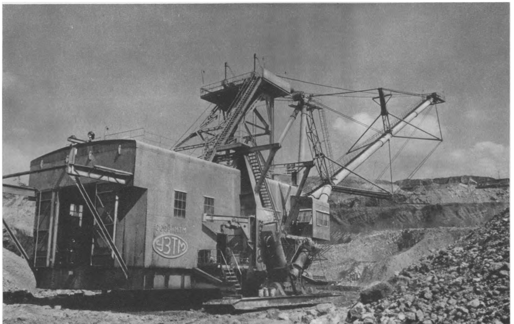
KARPINSK. A new power shovel in operation at the Vakhrushev fields in the Northern Urals, where opencut coal mining is widely practised. This is a walking-excavator model with a 10-cubic-metre bucket and 75-metre boom
