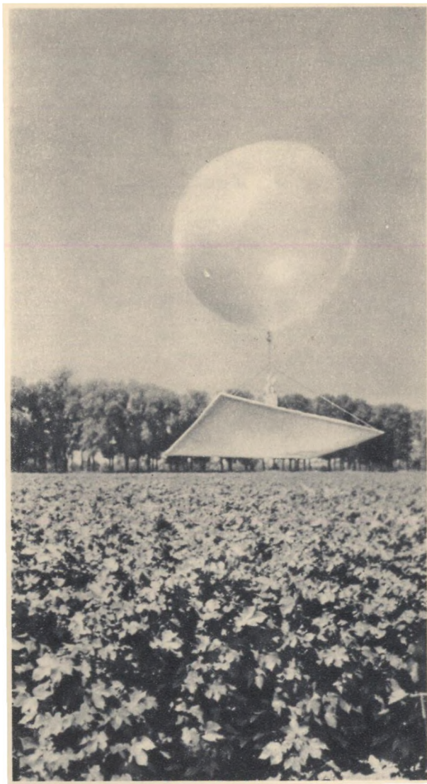
An equilibrated pilot balloon floats over a cotton field, showing the speed and direction of air currents
