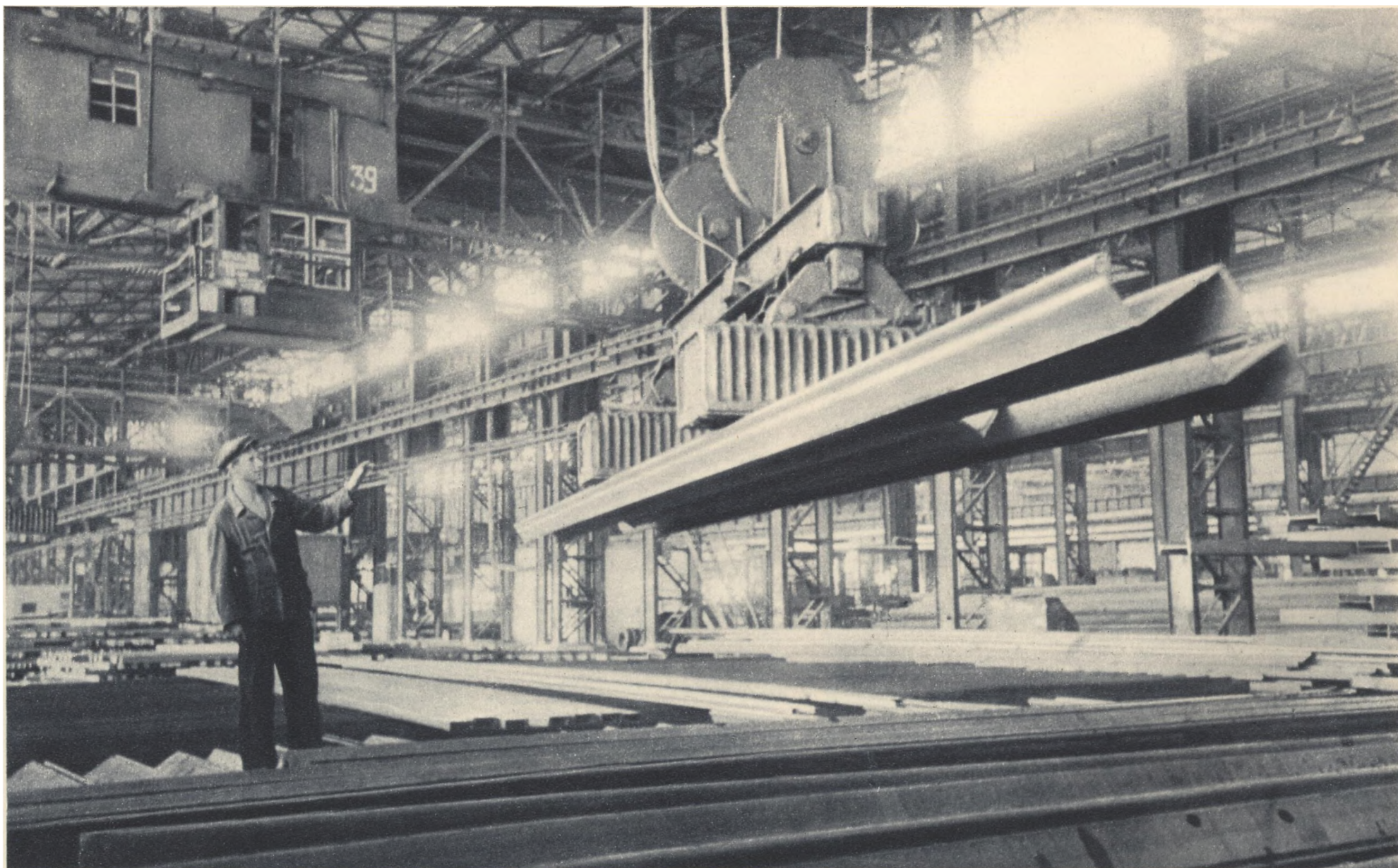
ZHDANOV (Southern Ukraine). The Azov Steel Mill is working on new orders from the great construction projects for sheet piles
