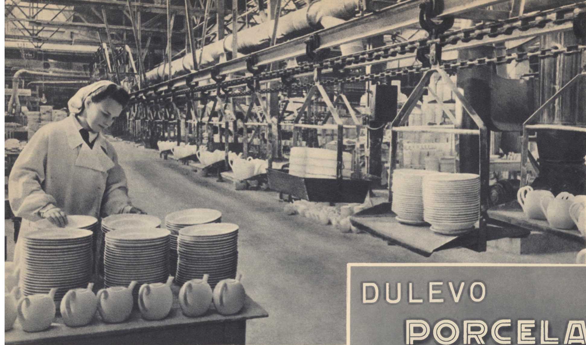
The transporter installed at the Dulevo Porcelain Works conveys the fabrics straight to the tunnel oven shop
