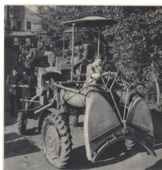
MOSCOW. One of the first self-propelled tea-plucking machines the production of which was recently begun at a Moscow factory. They will facilitate mechanization of the country's tea plantations. The machine gathers as many as 90 kilogrammes (198 pounds) in one hour Photographed by M. Ananyin
