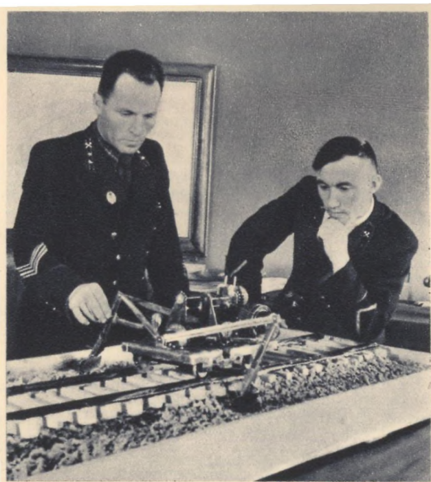
There are many inventors and rationalizers among the personnel of the Balkhash plant and mine. This picture shows A. Nesterov, chief of the technical department, examining a model of a scraper ballasting machine designed by technician A. Provtorov (right). The machine is intended for the placing of ballast in the construction of railway lines in the openworks
