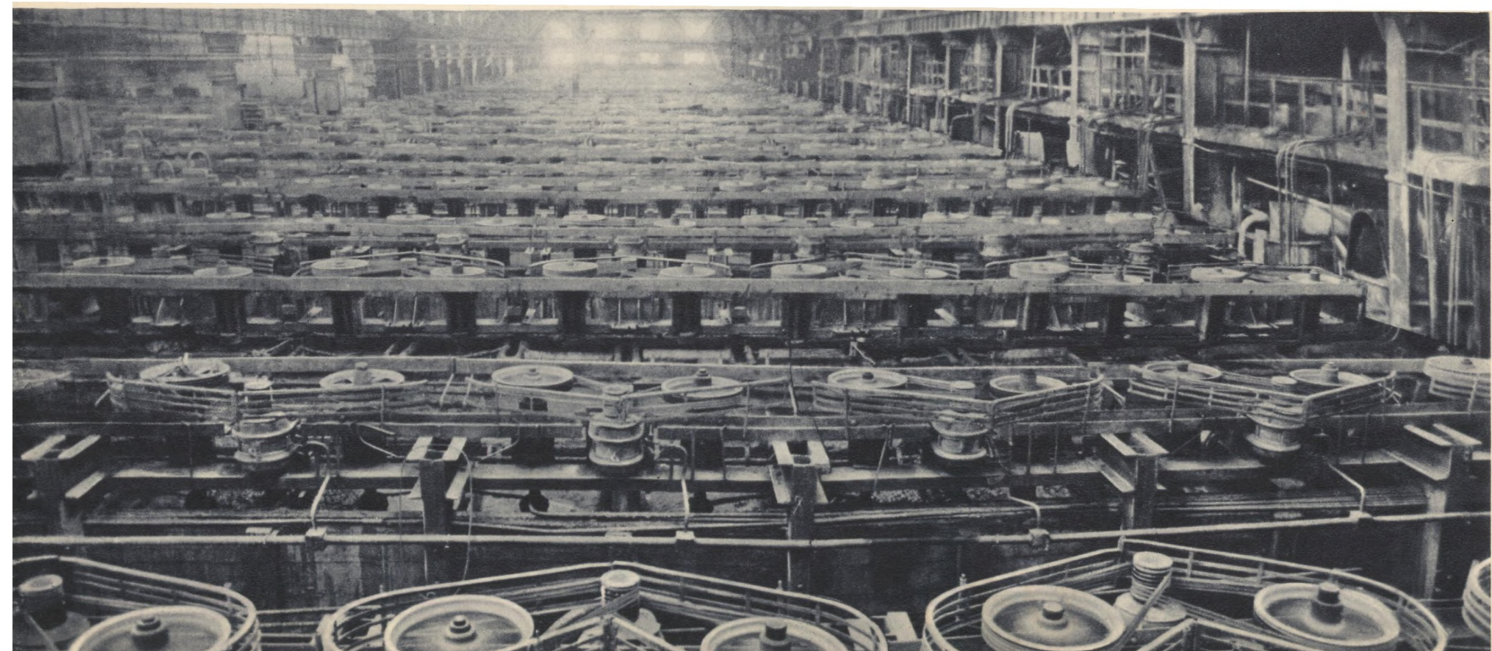
This is the flotation department of the concentration mill, where special machines eliminate extraneous substances from the ground ore
