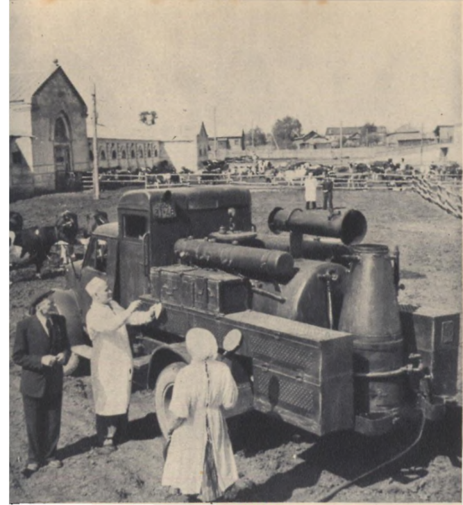
One of the Institute's professors, N. M. Komarov (centre) has designed a mobile machine which disinfects livestock premises and exterminates blood-sucking insects with a minimum expenditure of effort
