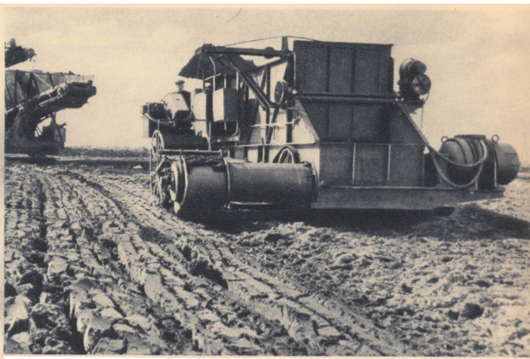
An electric spreading machine in the peat fields at Olaine. Soviet Latvia possesses vast peat resources which are mainly worked by machines
