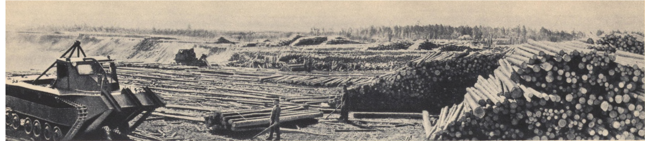
An amphibious tractor-winch rolls logs into the river Oyat at the Yarovshchina timber yard in Leningrad Region
