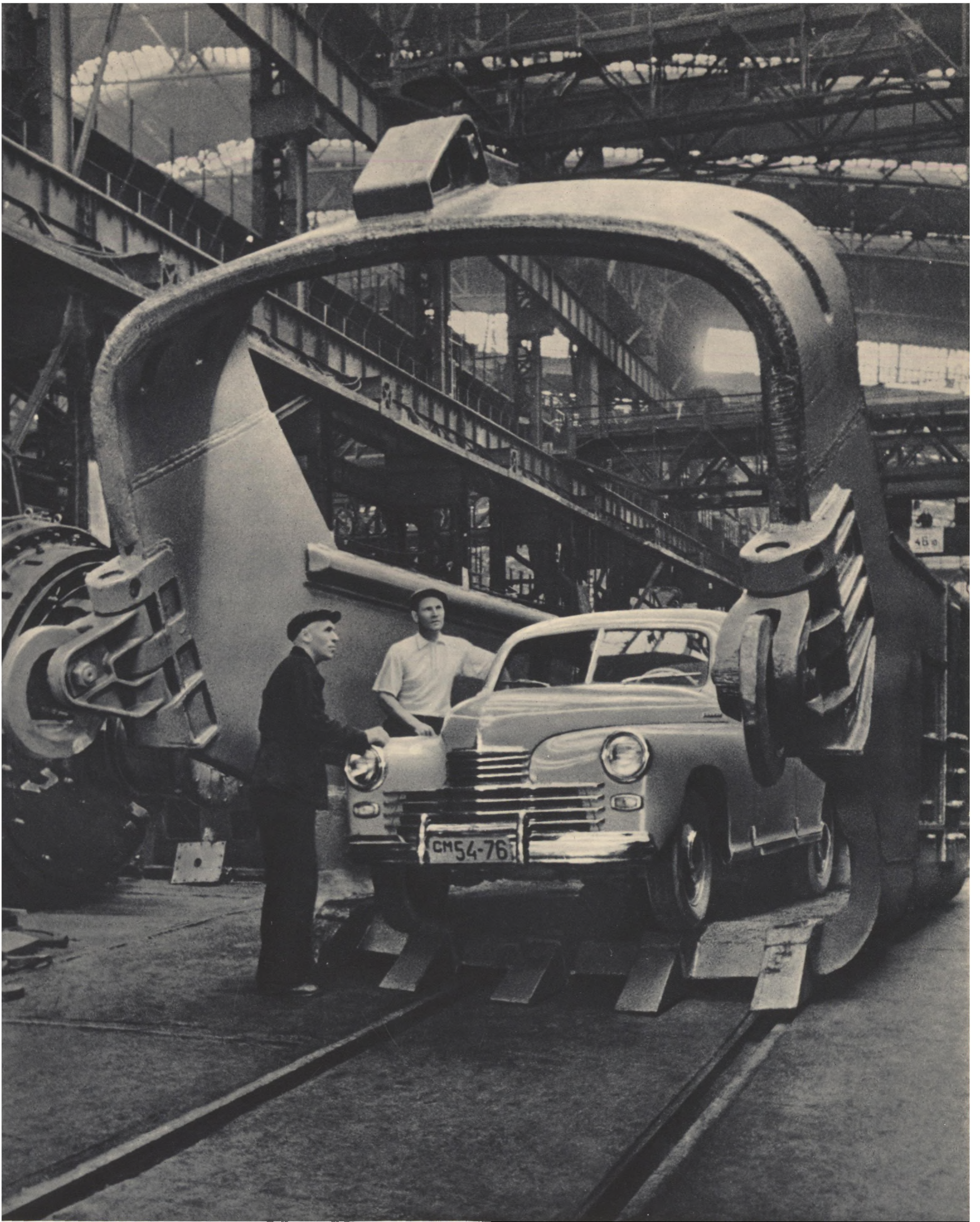
Twenty cubic metres (705 cu. ft.) of earth can be scooped up at one time by this bucket of walking excavator made recently at the Urals Heavy Machinery Works. The Pobeda car standing inside the bucket gives an idea of its dimensions. The walking excavator with a bucket capacity of 20 cubic metres is one of the new, super powerful excavating machines built to meet the further rapid development of the Soviet Union's coal mining industry and the increasing scope of construction work generally. In one minute this giant mechanical shovel can bring up earth from a depth of 35 metres (115 ft.), move it a distance of 120 to 130 metres (about 400 to 425 ft.) and return the bucket to the cut. In one hour it can shift about 1,200 tons of earth, or enough to fill approximately 250 five-ton lorries
