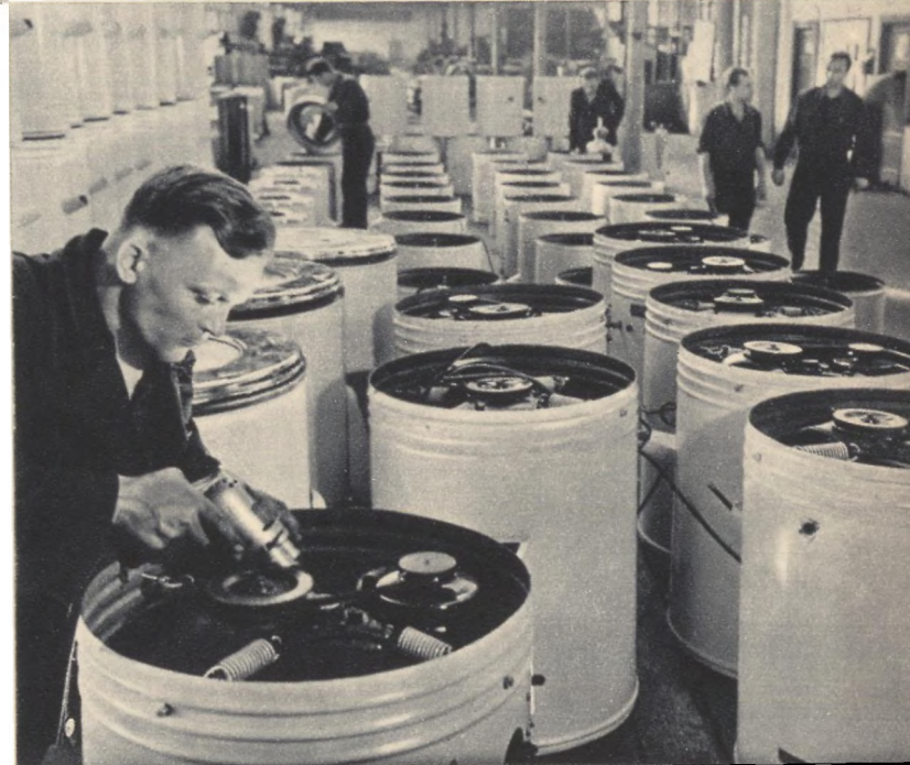
Assembly of electric washing machines at the REZ Electrical Engineering Works in Riga
