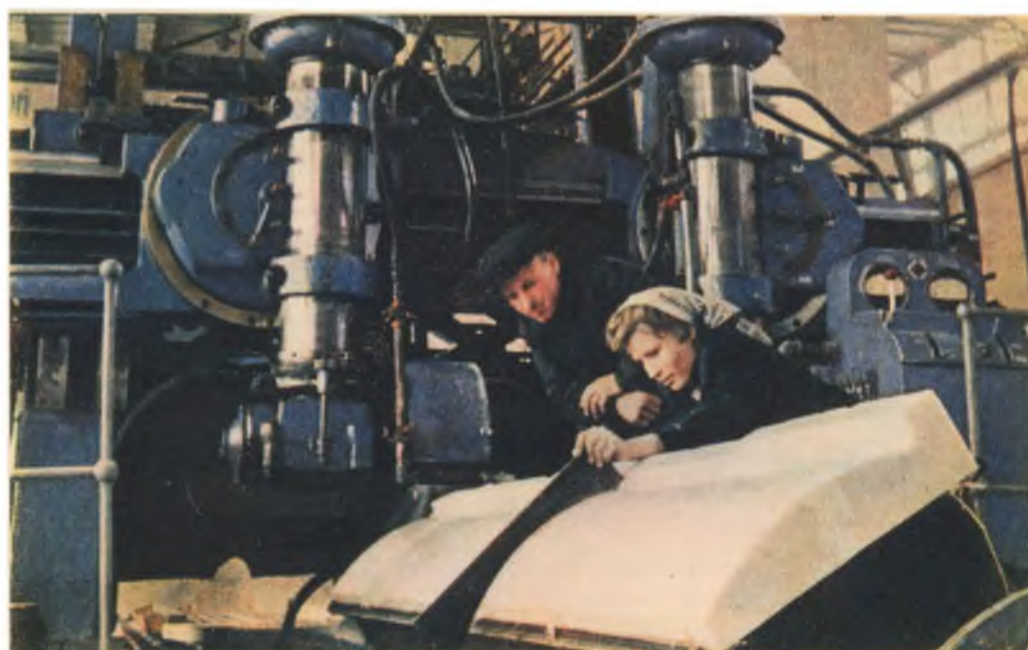
An operator checks the profile of a marble detail machined on a universal miller in a stone-working factory near Moscow
