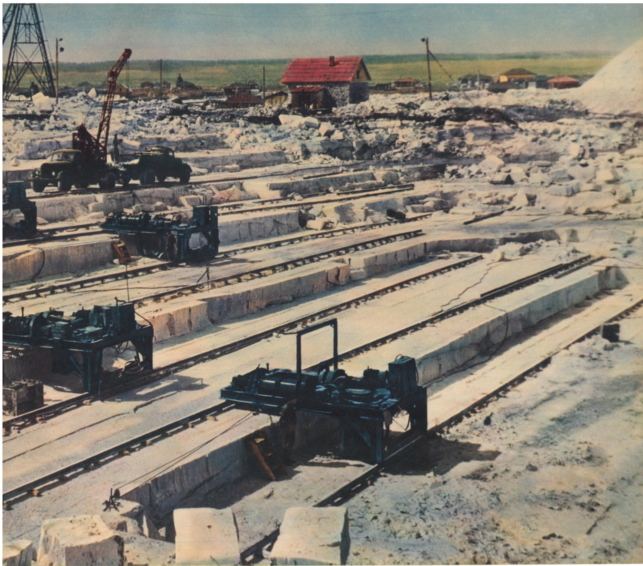
OM-177 stone-cutting machines, designed by A. Stolyarov, operating at the Koelga Marble Quarry in the Urals. Many Soviet marble quarries are now equipped with these machines which cut square blocks directly out of the mass
