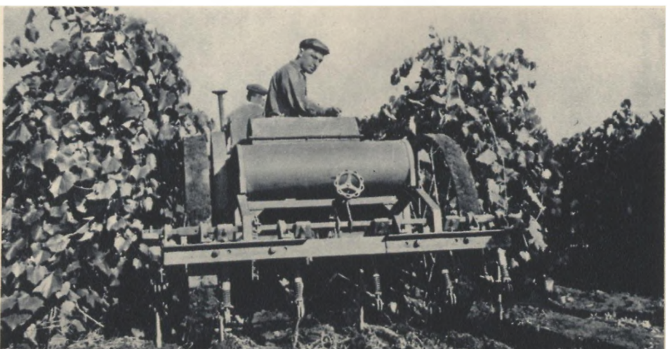
A tractor-drawn machine for treating the soil to a depth of eight inches
