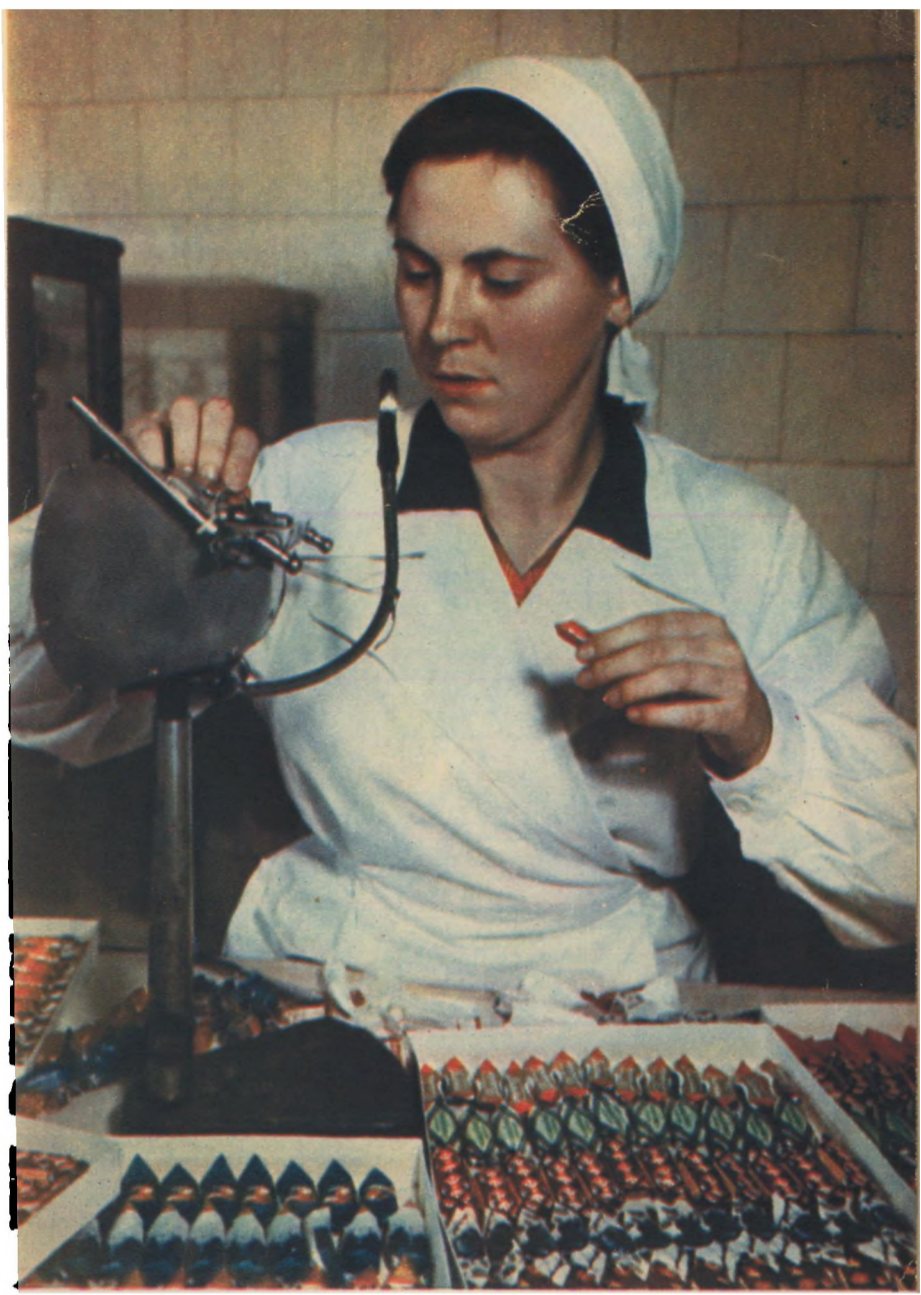
Margarita Minina, technologist in the assorted sweets department, gives a sweet filling a humidity test, to see that the factory's strict standard requirements are satisfied
