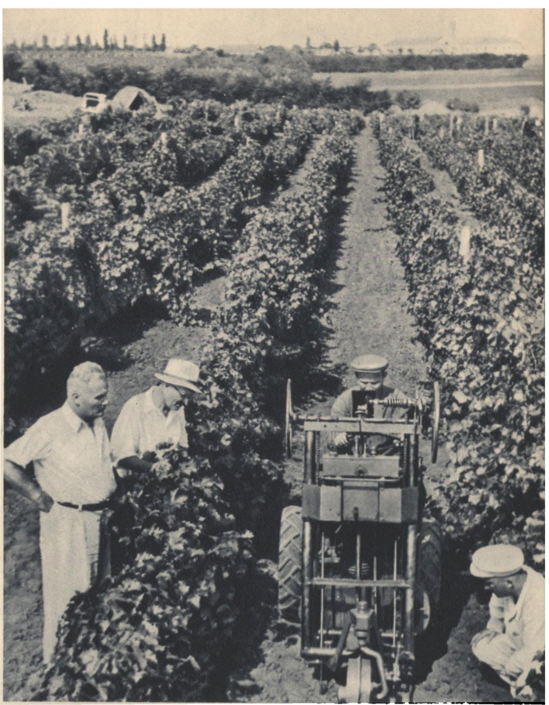
A self-propelled machine for deep impregnation of the soil at work at the Grateshti State Farm, Kishinev District. Anti-phylloxera preparations are injected into the ground at depths of 8, 24, and 40 inches. As a result the vine-lice are destroyed and the vine remains undamaged
