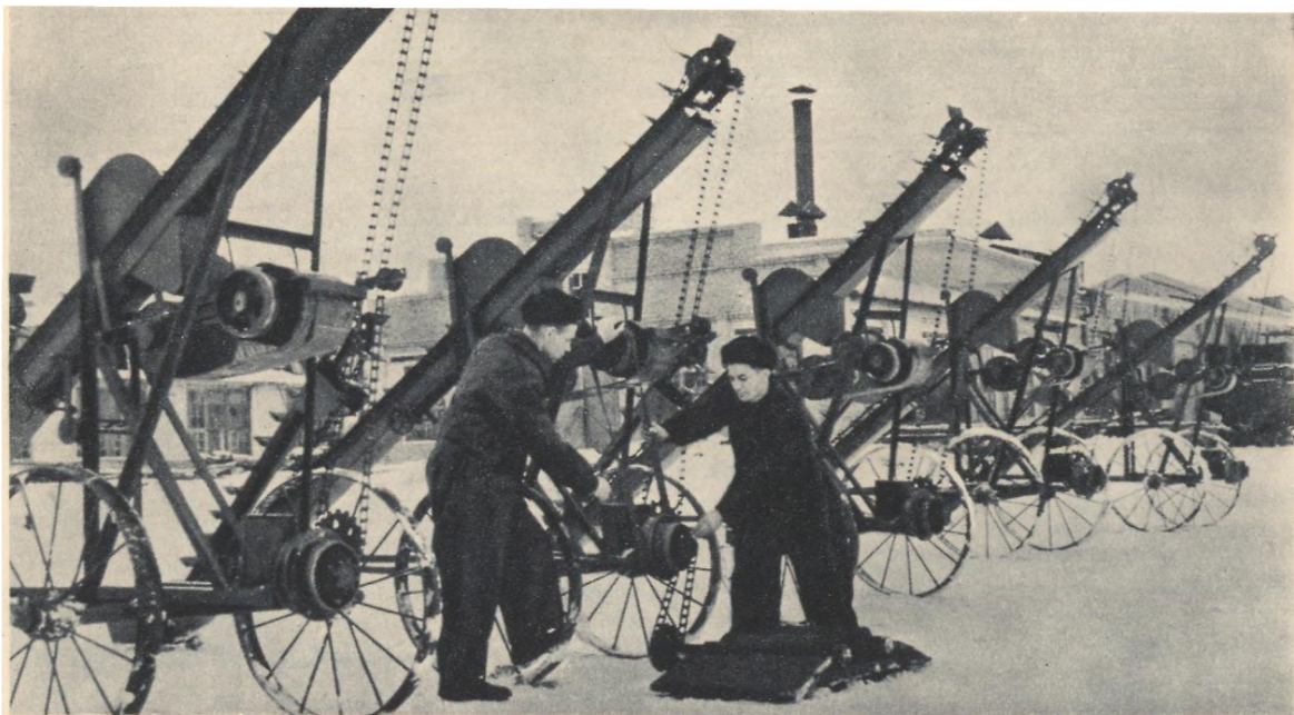
STALINGRAD. The Motor-Repair Works puts out these grain-loaders. Driven by a motor-car engine, they handle 18-20 tons of grain an hour. The production programme of the works has been doubled for 1954 Photographed by A. Makletsov
