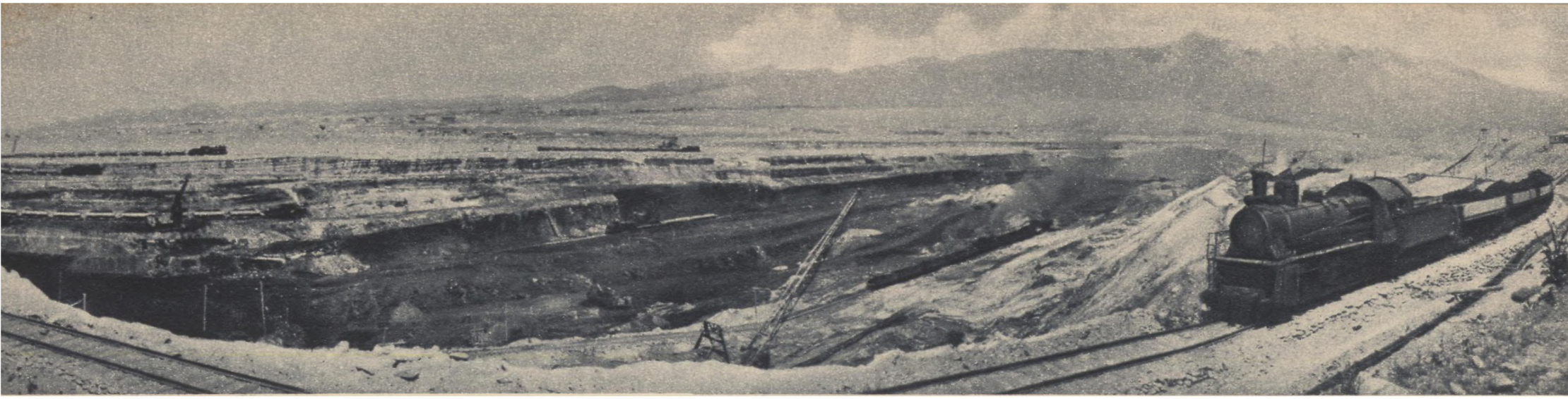
A view of the Angren open-cut working. Electric excavators strip the cover and remove the coal
