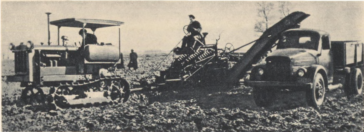
KIEV REGION. This is an improved three-row beet-harvesting combine, SKEM-3, designed by V. A. Korenkov, a Stalin Prize winner Photographed by S. Ostrovsky
