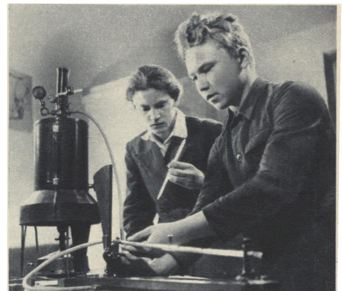
In the physics lab two pupils, Yuri and Boris, are engaged in a thrilling experiment. They are determining the coefficient of linear expansion
