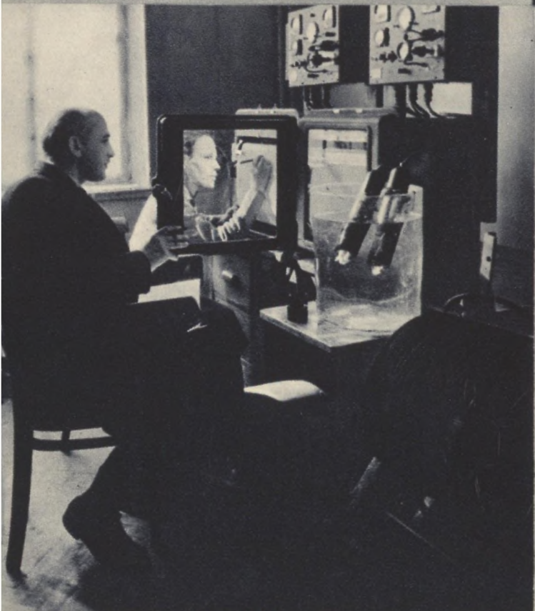
New precise methods of measuring physical magnitudes are being used in the most unexpected quarters. They have penetrated every branch of modern engineering and are now invading navigation. The picture shows V. Novish and O. Gorodnicheva improving an electromagnetic sea current meter. This simple device makes it possible to determine the speed of a current without slowing down a ship
