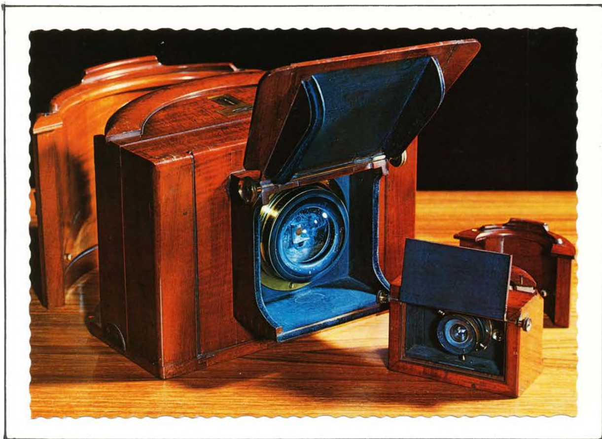
Thomas Sutton panoramic Cameras: With Cox water lens 1859. With Ross water lens 1861. Foto: Preus Fotomuseum. Horten.
