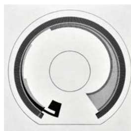
FRE, Functional Resistor Element.
